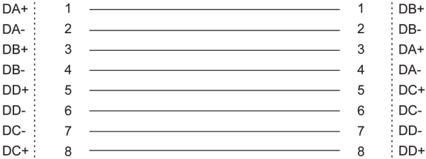
Straight-through Cable Wiring (MDI to MDI-X)
