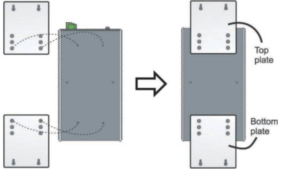
**STEP 2**—Mounting the EDS-P510 on the wall requires 4 screws. Use the EDS-P510, with wall mount plates attached, as a guide to mark the correct locations of the 4 screws. The heads of the screws should be less than 6.0 mm in diameter, and the shafts should be less than 3.5 mm in diameter, as shown in the figure on the right.
