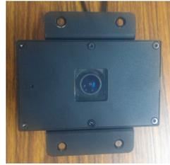
**Step 2: Use the installation sticker to drill the holes for flush-mounting the VPort P06HC with the VP-FD1.**
