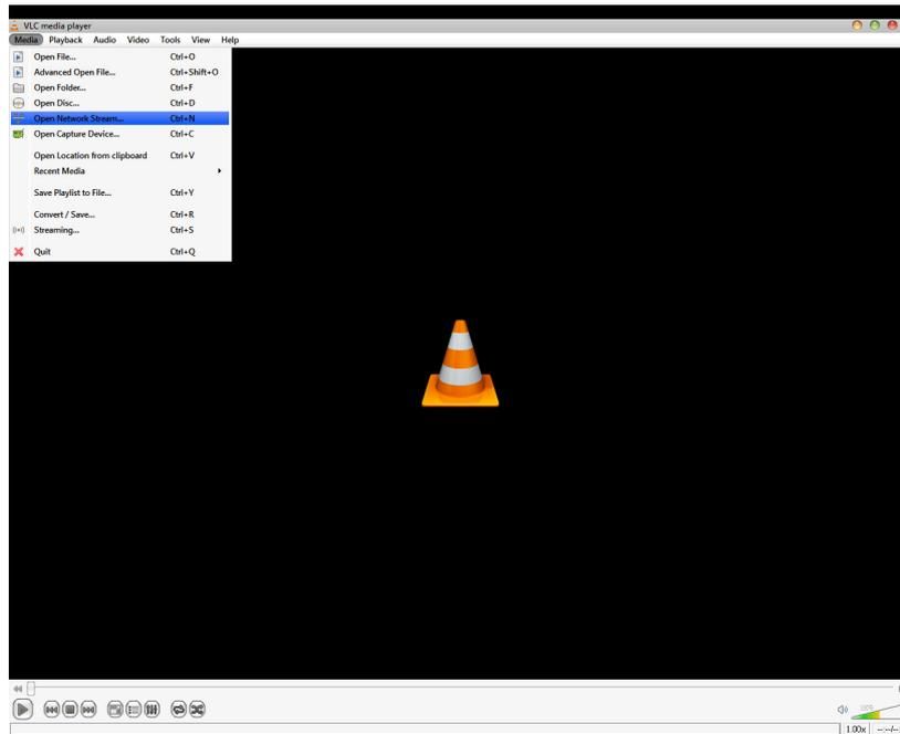
**Step 2:** When the following pop-up window appears, type the URL in the input box. E.g., type **rtsp://<VPort P06HC-1MP-M12's IP address>[:<RTSP Port>]/udpstream\_ch1\_stream< 1 or 2>**
