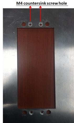
**NOTE** The screw holes for mounting the 2 VP-FD1's mounting kits are countersunk holes with 8 mm top diameter and 4.3 mm chamfer. Take this into consideration when drilling these 4 screw holes.
