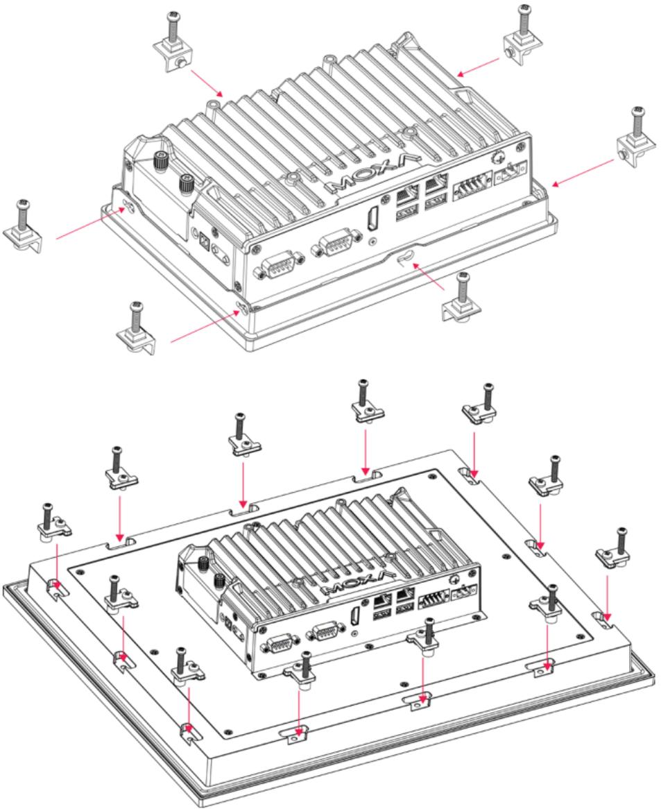
Use a torque of 5 kgf-cm to secure the mounting screws to fasten the panel-mounting kit onto the wall.
