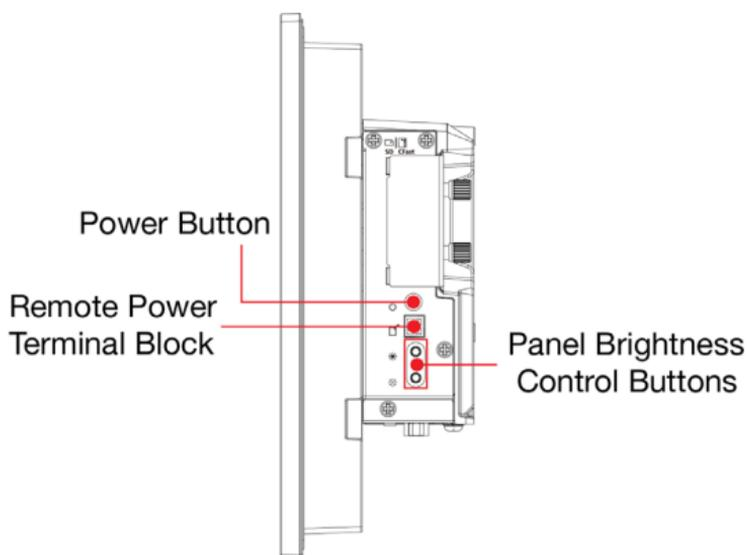
The display-control buttons can be used as described in the following table:
