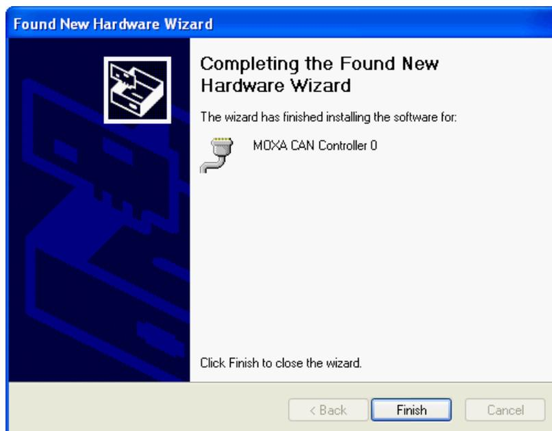
**Step 5:** Repeat Step 1 through Step 4 for each of the remaining controllers (note that there are 2 controllers for a 2-port board).
