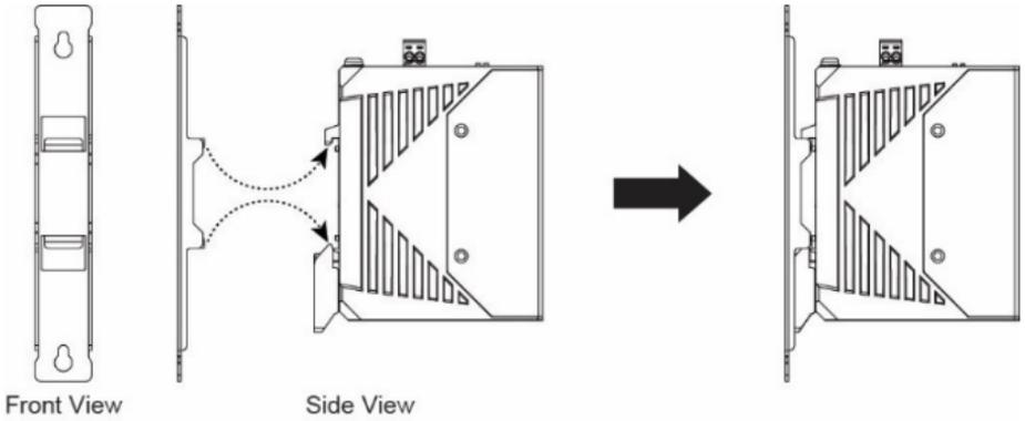
There are two options for installation: The first option is to hook the EDS DIN-rail latch on the opening of the wall mount kit (see picture above) and then mount the wall-mount kit on the wall with screws. (The other option is to perform these two steps in the other order.) The heads of the screws should be less than 6.0 mm in diameter, and the shafts should be less than 3.5 mm in diameter, as shown in the figure at the right.
