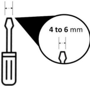
Please use a flat-head screwdriver with a head size of between 4 and 6 mm for proper installation or removal.
