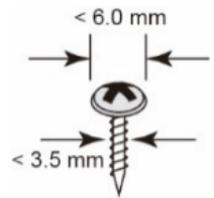
**NOTE** Before tightening screws into the wall, make sure the screw head and shank size are suitable by inserting the screw into one of the keyhole-shaped apertures of the Wall Mounting Plates.
