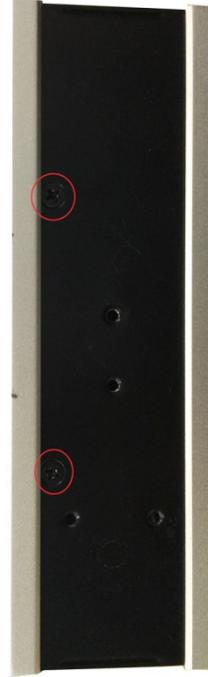
3. Remove the four screws on the silver cover on the right panel and take off the cover.
