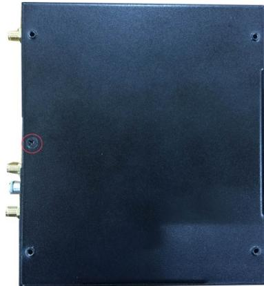
5. Remove the three screws on the top panel.
