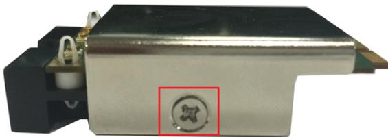
13. Insert the module into the socket and secure it using a screw from the package.
