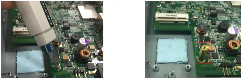
10. Attach one thermal pad to the cellular module cover and the other thermal pad to the module pad.
