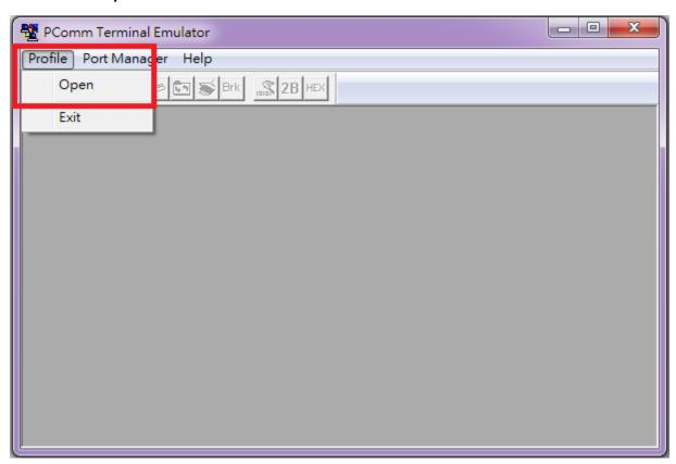
5. Specify which COM port is connecting to the Moxa controller, and then use the following configuration settings: 115200, 8, none, 1.
