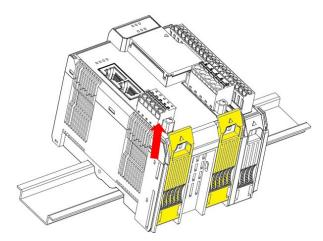
**Step 2:** Press the release tab (item 1 in the figure) and then remove the CPU module from the DIN rail (item 2 in the figure).
