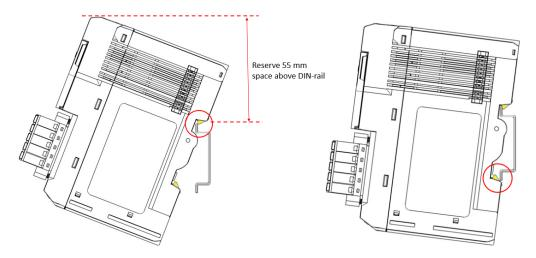
Step 2: Push the unit towards the DIN rail until the end of the mounting clip snaps into place.
