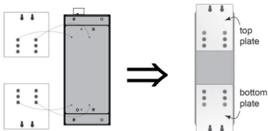
**STEP 2:** Mounting the OBU-102 on the wall requires 4 screws. Use the switch, with wall mount plates attached, as a guide to mark the correct locations of the 4 screws. The heads of the screws should be less than 6.0 mm in diameter, and the shafts should be less than 3.5 mm in diameter, as shown in the figure at the right.
