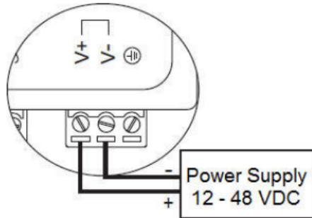
The TCC-100 is powered by an external 12 to 48 VDC power supply. To connect the power supply, run two wires from the V+ and V- terminals on the TCC's 3-connector terminal block to the DC power supply, as shown in the figure. Once the power supply is connected to its power source, the PWR LED located on the TCC's top panel should turn red.
