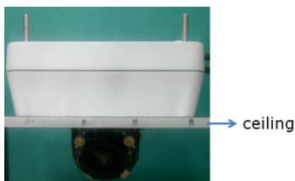
**Step 5: Loosen the screws that fix the horizontal and vertical lens positions. Next, tune the camera lens position, and connect to the VPort P16's web console to view the video image. After the lens position is correct, fix the screws (5.5 kgf-cm torque is required).**
