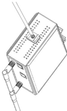
**STEP 2:** After mounting the AWK-3262A and plugging in the LAN cable, tighten the cable along the device and wall.
