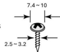
**NOTE** Test the screw head and shank size by inserting the screws into one of the four screw holes of the wall-mounting plates before they are fixed to the wall.
