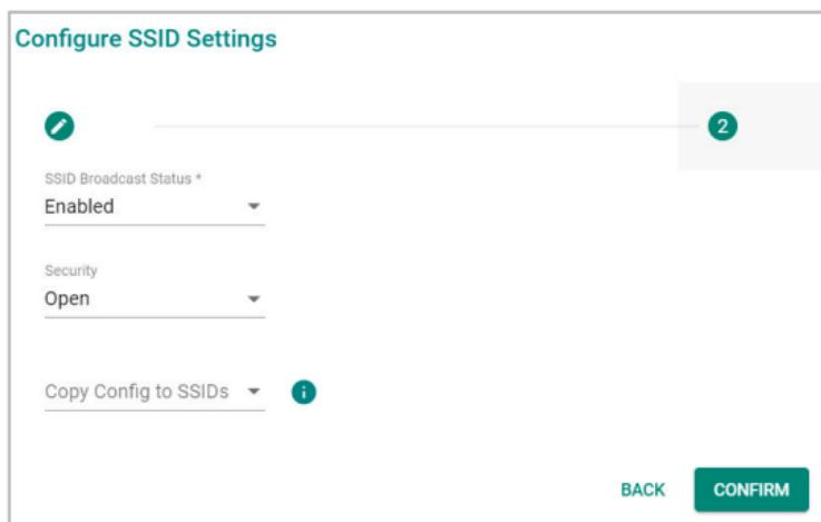
This screenshot shows the 'Configure SSID Settings' screen for the second SSID. It includes fields for SSID Broadcast Status (Enabled) and Security (Open). A 'Copy Config to SSIDs' button is at the bottom. At the bottom right are 'BACK' and 'CONFIRM' buttons.
