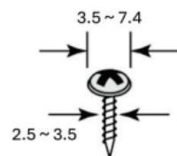
Do not drive the screws in all the way—leave a space of about 2 mm to allow room for sliding the wall-mounting panel between the wall and the screws.
