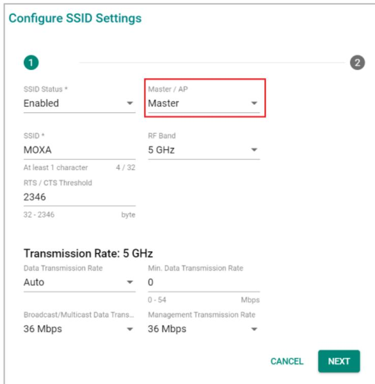
This screenshot shows the 'Configure SSID Settings' screen for the first SSID. It includes fields for SSID Status (Enabled, Master selected), SSID name (MOXA), RF Band (5 GHz), RTS / CTS Threshold (2346), and a transmission rate section for 5 GHz. The 'Transmission Rate: 5 GHz' section contains dropdowns for Data Transmission Rate (Auto, 0 Mbps), Broadcast/Multicast Data Trans... (36 Mbps), and Management Transmission Rate (36 Mbps). At the bottom are 'CANCEL' and 'NEXT' buttons.
