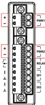
**STEP 1:** Insert the negative/positive DC wires into the +/- terminals.
