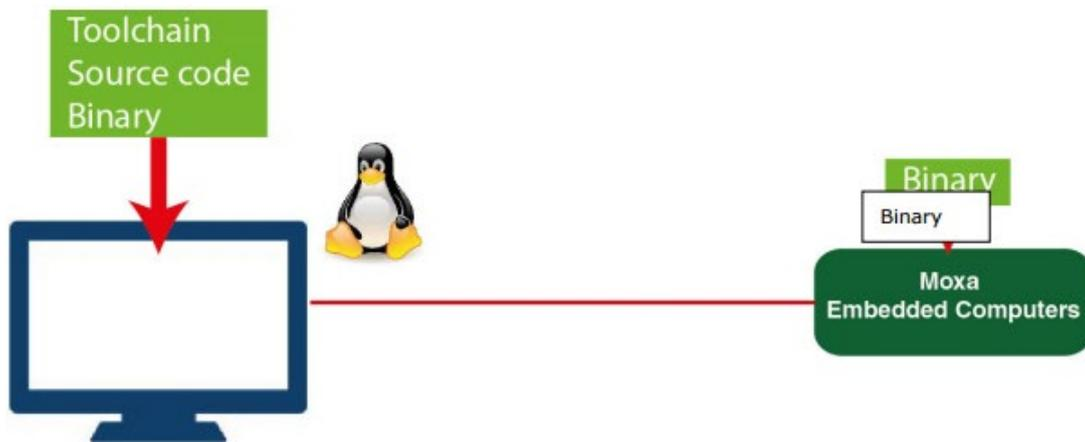
To ensure that an application will be able to run correctly when installed on Moxa computers, you must compile the application and link it to the same libraries that will be present on Moxa computers. This is particularly true when the Arm-based Cortex processor architecture differs from the CISC x86 processor architecture of the host system, but it is also true if the processor architecture is the same.
