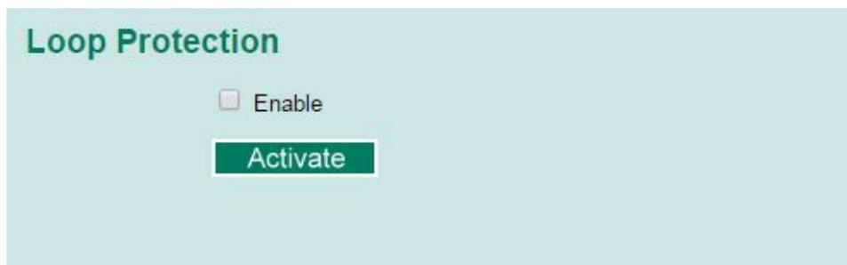
Check the Enable box and click Activate to enable the Loop protection.
