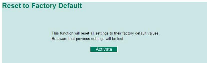
This function provides users with a quick way of restoring the Moxa switch’s configuration to factory defaults. The function is available in the serial, Telnet, and web consoles.
