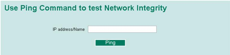
The **Ping** function uses the *ping* command to give users a simple but powerful tool for troubleshooting network problems. The function’s most unique feature is that even though the ping command is entered from the user’s PC keyboard, the actual ping command originates from the Moxa switch itself. In this way, the user can essentially sit on top of the Moxa switch and send ping commands out through its ports.
