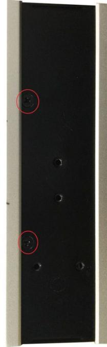
3. Remove the four screws on the silver cover on the right panel and take off the cover.
