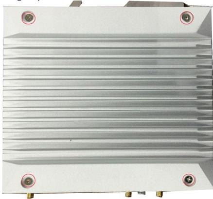
4. Remove the screw on metal cover.
