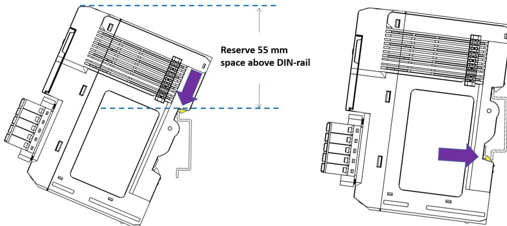
**Step 2:** Push the unit towards the DIN rail until the end of the mounting clip snaps into place.
