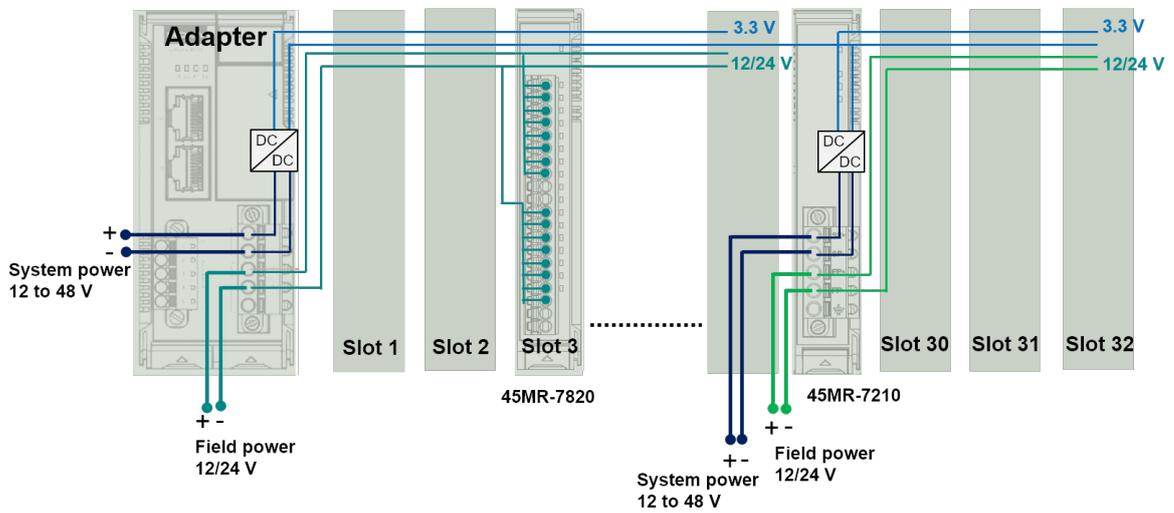
**NOTE** All I/O points have 3 kV VDC or 2 kVrms isolation with the system. We recommended using different power supplies to ensure that the system power and field power are isolated from each other.
