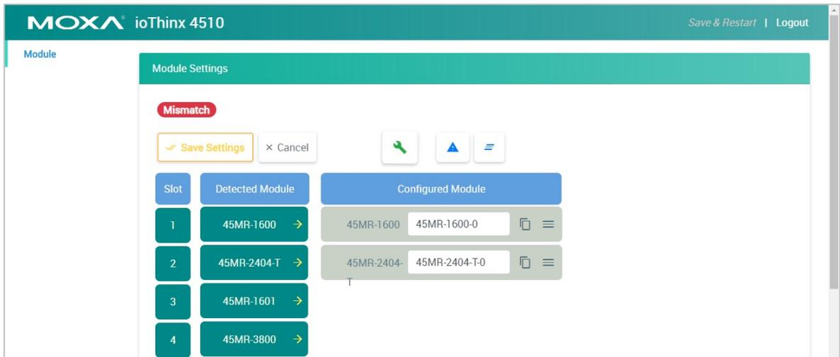
In edit mode, if any detected modules and configured modules do not match, then the configured modules will be highlighted as shown below.
