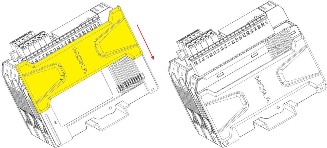
**NOTE** The covers provide protection against electrostatic discharge.
