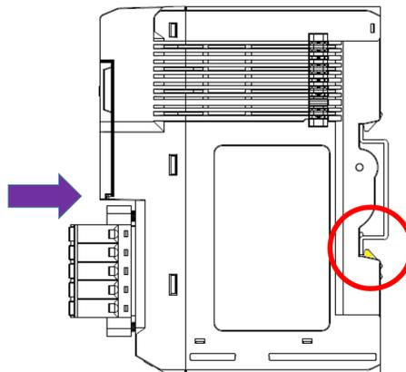
**INFORMATION** When the I/O module is inserted into the correct position, the connection between the internal bus and the previous module is established.
