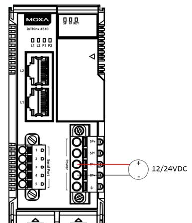
**NOTE** The 12/24 VDC field power supply can be connected directly to 45MR modules. If more connection points are needed, purchase 45MR-7820 (8 x FP+ and 8 x FP-) modules.
