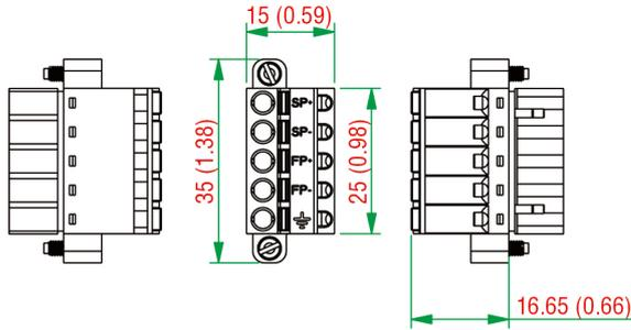
The device requires two sets of power inputs. One is for the system (internal logic circuit), and the other is for field I/O circuits.
