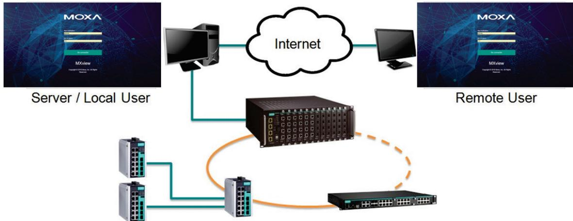
The MXview server runs in the background on a Windows PC and communicates with network devices using Simple Network Management Protocol (SNMP) and a Moxa proprietary protocol that periodically polls specific MIB data and stores data in a local database.
