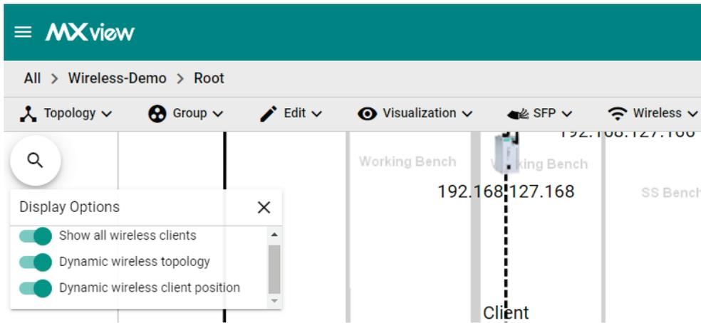
The following diagrams are an example of the dynamic roaming display showing dynamic client-AP link changes.
