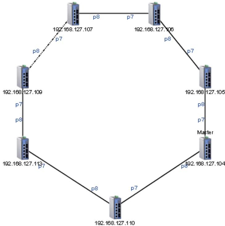
For devices that play a particular role in the topology, MXview will label the devices by displaying the roles above the images of the devices. Backup links will be indicated with dashed lines.
