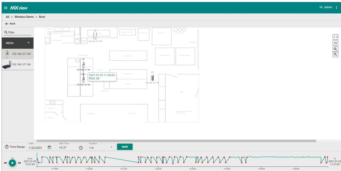
On the left-hand side is a list of wireless clients, in the center is the topology map, and located at the bottom is the playback progress bar. Select any client from the list and click **Play** (▶) to start playing the wireless roaming history for the selected time range. You can adjust the playback speed by clicking the **Decrease Speed** (◀◀) or **Increase Speed** (▶▶) button to increase or decrease the playback speed respectively.
