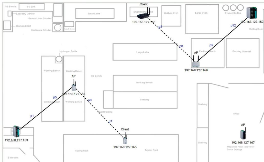
When the client roams to another AP, MXview will automatically redraw the link to the new AP on the wireless topology diagram.
