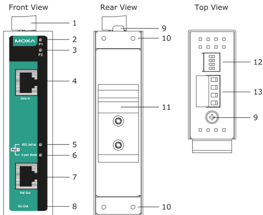
1. Terminal block for P1/P2 power inputs
