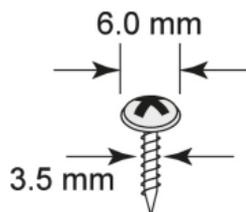
**NOTE** Before tightening the screws into the wall, make sure the screw head and shank size are suitable by inserting the screw into one of the keyhole-shaped apertures of the wall mounting plates. Do not tighten the screws completely—leave about 2 mm to allow room for sliding the wall mount panel between the wall and the screws.
