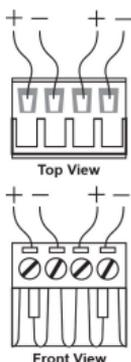
**STEP 1:** Insert the negative/positive DC wires into the V-/V+ terminals.
