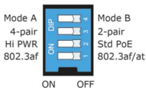
The default setting for each DIP switch is OFF. The following table explains the effect of setting the DIP switches to the ON positions.
