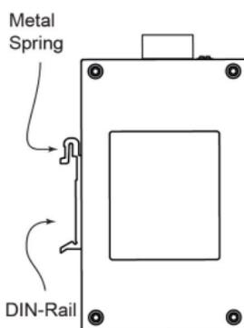
To remove the INJ-24A from the DIN rail, simply reverse steps 1 and 2 above
