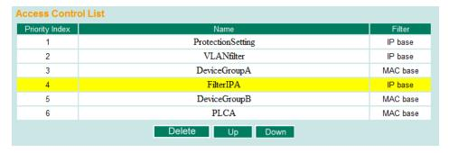
Changing an established access control list's priority is easy. Moxa provides a simple interface to let you easily adjust priorities. Follow the three steps below to adjust the priority:
