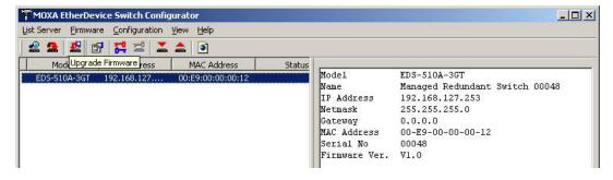
3. Click the **Upgrade Firmware** toolbar icon , or select **Upgrade** under the **Firmware** menu. If the switch is Locked, you will be prompted to input the switch's Username and Password.
