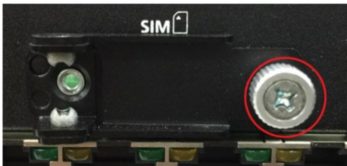
2. Insert the SIM card into the slot. Make sure you insert the card in the direction indicated above the card slot.
