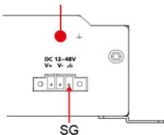
**SG:** The Shielded Ground (sometimes called Protected Ground) contact is the right most contact on the 3-pin power terminal block connector when viewed from the angle shown here. Connect the SG wire to an appropriate grounded metal surface. An additional ground connector is provided just above the power terminal block, which you can use for grounding protection.
