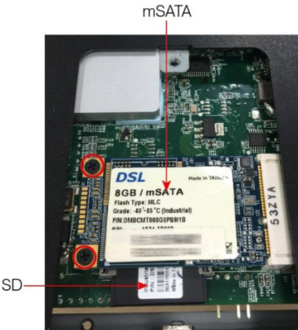
3. Push the SD card in gently to release it and remove the SD card to insert a new one in the socket. Make sure your SD card has been securely inserted.
