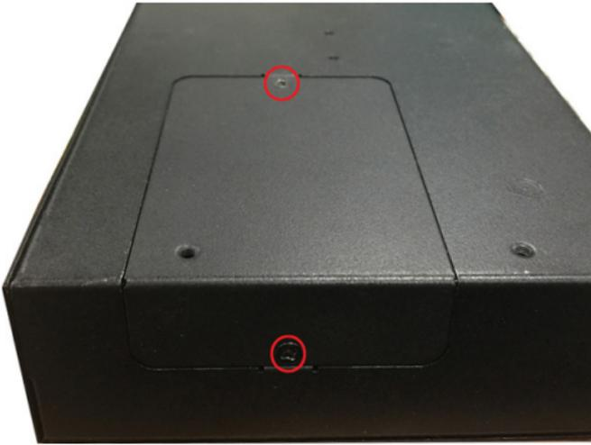
2. Remove the cover to access the SD-card slot and the mSATA socket.
